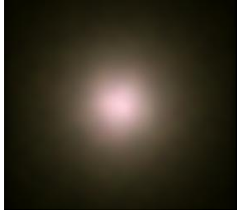
TracePro TrueColor Irradiance Map raytrace at a 2.2cm distance
