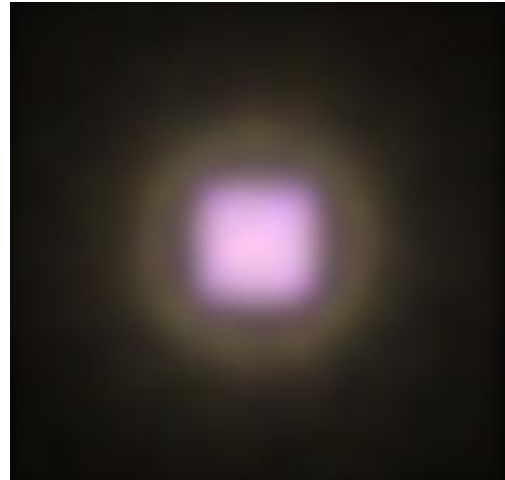
TracePro TrueColor Irradiance Map raytrace at a 10cm distance
